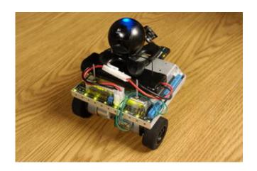
Qwerkbot, a three-wheeled robot that can send images over the Internet, is one of several robots that can be built with the Telepresence Robot Kit (TeRK), a combination of a robot controller, commonly available parts and assembly instructions (recipes) developed by the CREATE Lab in Carnegie Mellon University&acutes Robotics Institute. Photo credit: Ken Andreyo/CMU
