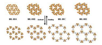
Structures (along the c axis) of the MIL-88A, B, C, D series in their dry forms (top) and open forms (bottom). Credit: Institut Lavorsier
