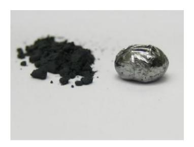
UCLA scientists have made rhenium diboride, an "ultra-hard material." Rhenium diboride is seen here in powder form (left), made from heating the elements in a furnace, and as a pellet made by a procedure called arc melting. Credit: UCLA
