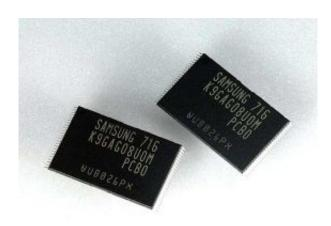
Samsung Electronics announced today that it has become the first to begin mass producing 16 gigabit NAND flash, the highest capacity memory chip now available. The company said it will fabricate the devices in 51 nanometers, the finest process technology to be used in memory mass production to date.
