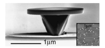
Microdisk lasers used in experiments by NIST, Stanford University and Northwestern University are made by layering indium arsenide on top of gallium arsenide and etching out disks about 1.8 micrometers across on pillars of gallium arsenide. Scanning tunneling microscope image (inset) shows some of the approximately 130 "quantum dot" islands of indium arsenide in each disk. Credit: NIST
