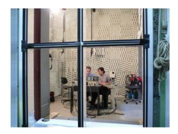
Students measure the vibrations in the frame of a noise-absorbing window. The walls are cladded with soundproof material to prevent noise from being propagated. © SzM Technische Universität Darmstadt
