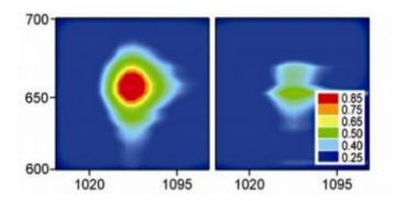
Biomedical applications could exploit the natural fluorescence of the carbon nanotubes. When light is polarized along a single-walled carbon nanotube (left), this fluorescent emission is strong. Credit: NIST
