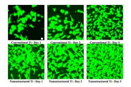
The faster endothelial cells (green) form a single smooth layer, the less chance exposed metal will provoke an immune response. Samples examined after 1, 3 and 5 days (left to right) show better coverage on nanotextured titanium (bottom row) than on conventional microstructured titanium. Credit: Image: Thomas Webster
