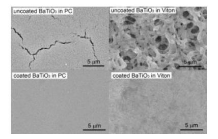
Scanning electron micrographs of barium titanate (BaTiO3) nanocomposites with polycarbonate (left, top and bottom) and Viton (right, top and bottom) polymer matrices. The images show the dramatic improvement in film uniformity through the use of phosphonic acid coated BaTiO3 nanoparticles (bottom images) as compared to uncoated nanoparticles (top images). Credit: Image courtesy of Joe Perry
