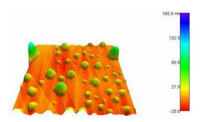
The green circles are the nanobubbles on a solid. The bubbles are about 10 nm high and 1000 nm across at the base. Credit: Xuehua Zhang
