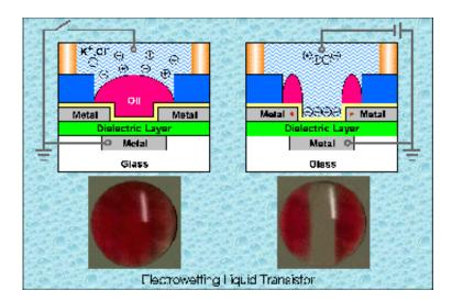
Diagram and photograph of red-tinted oil being separated by electric current. Credit: University of Cincinnati
