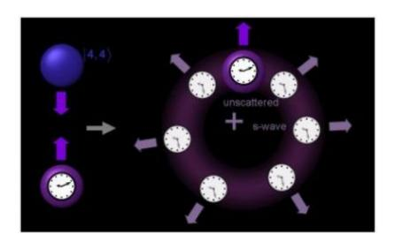
Schematic of the Experiment. We collide a clock atom with atoms in another state (labeled |4, 4>). When the clock atoms collide, they experience a discrete jump, which is the difference of two s-wave phase shifts. The s-wave phase shifts can be measured with atomic-clock accuracy and give precise information about the atom-atom interactions. Credit: Kurt Gibble, Penn State
