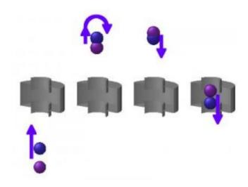
Schematic of Fountain Clock Juggling Cesium Atoms. Two clouds of cesium atoms are tossed upward with a short time delay so that they collide after passing through the microwave cavity (silver) on the way up and before they return down through the cavity. The microwaves in the cavity excite and probe the atoms, resulting in an atomic fountain clock. Credit: Kurt Gibble, Penn State
