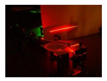
A microstructured optical fiber in NIST's new paired-photon source delivers high numbers of photon pairs over a broad bandwidth with low noise, all in a compact device for quantum communication devices. Credit: Migdall/NIST
