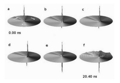
A graphical representation of the magnetization of a magnetic disk with a rotating vortex. **a-f**, Over a time period of about 20 nanoseconds, the magnetization of the core (represented by the spike in the center of the disk) moves circularly around the disk&acutes center. Simultaneously, the magnetization switches from upward to downward and begins to switch back to upward.
