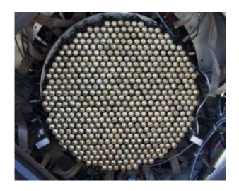
Iowa State University astrophysicists designed and built four of these cameras for the VERITAS gamma ray telescope system. Each camera contains 500 tube-shaped photo detectors. Credit: Photo contributed by Frank Krennrich/Iowa State University
