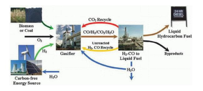
A possible configuration of the proposed H2CAR process. Image credit: Rakesh Agrawal, et al.
