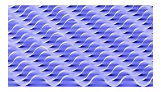
Semiconductor ribbons with buckled profiles on polydimethylsiloxane surfaces that are functionalized for surface chemical bonding exhibit mechanical stretchability. Credit: Argonne National Laboratory
