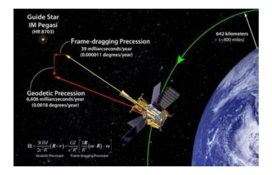
With its telescope aimed at IM Pegasi, a far-off guide star serving as a fixed reference point, the experiment measured tiny changes in the direction of spin of four gyroscopes. Credit: Stanford University
