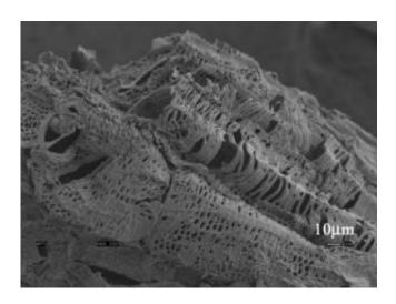
A magnified image of a cornstalk particle shows the many tiny pores that pretreatment -- a phase of the ethanol production process -- opens up. These pores create more surface area for subsequent reactions to take place and give enzymes better access to cellulose, the source for cellulosic ethanol. Researchers said this information could help in establishing an economic method for industrial production of cellulosic ethanol. Credit: Purdue University photo/Meijuan Zeng
