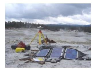
Sitting on a tripod, a Global Positioning System (GPS) antenna, powered by portable solar-energy panels, measures gradual movements of Earth's crust in Hot Springs Basin, Yellowstone National Park, Wyoming. University of Utah researchers have published 17 years worth of GPS data showing how a giant plume of hot and molten rock beneath Yellowstone shapes the landscape of the park and a wide area around it. Credit: Jamie Farrell, University of Utah
