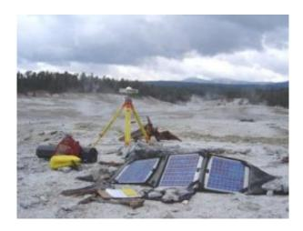
Sitting on a tripod, a Global Positioning System (GPS) antenna, powered by portable solar-energy panels, measures gradual movements of Earth's crust in Hot Springs Basin, Yellowstone National Park, Wyoming. University of Utah researchers have published 17 years worth of GPS data showing how a giant plume of hot and molten rock beneath Yellowstone shapes the landscape of the park and a wide area around it. Credit: Jamie Farrell, University of Utah
