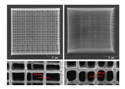
Scanning electron microscope images of woodpile-type photonic crystal structures fabricated with 520 nanometer excitation at (a) higher power and at (b) lower power using DABP. Magnified images of the structures are shown below their respective overview images. Credit: Wojciech, H. et al.
