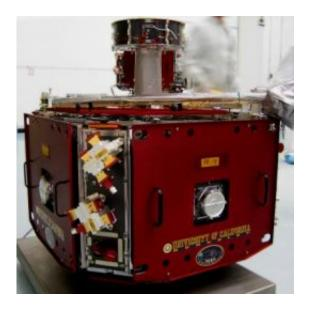
One of the five THEMIS spacecraft prior to launch. Its two solid-state telescope units, each with two opposite-facing SSTs incorporating four silicon detectors each, are mounted on the near edge. Credit: UC Berkeley Space Sciences Laboratory
