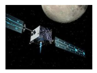
Artist's impression of ESA's SMART-1 mission at the Moon. SMART-1 was launched in September 2003, and arrived to the Moon on 15 November 2004, after a long spiralling around during which it tested new technologies, including solar-electric propulsion for future applications in interplanetary travels. The mission ended through lunar impact on 3 September 2006. Credits: ESA - AOES Medialab
