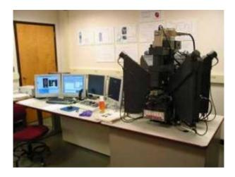
Using the custom-built Ultrachron, UMass Amherst scientists are assigning dates to the geologic processes that rocks experience with new precision. Credit: University of Massachusetts Amherst
