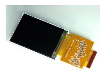
Samsung Electronics announced today that it has developed a 2.1" LCD panel for high-end mobile devices that will provide qVGA resolution and comes equipped with sensors designed to adjust brightness to optimize ambient lighting. Screen brightness is automatically adjusted to enhance readability under any lighting condition.
