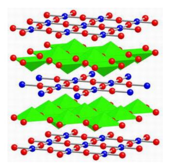
Diagram shows the typical T&acute structure of PLCCO superconductors, consisting of CuO2 sheets separated by thin sheets of rare-earth oxide. Credit: Argonne National Laboratory
