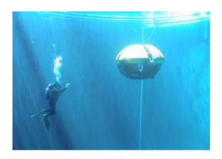
Doctoral student Marcus Gary SCUBA dives with the DEPTHX probe during initial in-water tests at The University of Texas at Austin Applied Research Laboratories wet test facility.
