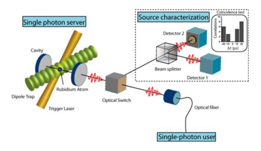
A single atom trapped in a cavity generates a single photon after being triggered by a laser pulse. After the source is characterised, the subsequent photons can be distributed to a user. Image: Max Planck Institute of Quantum Optics
