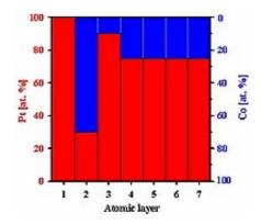
Segregation profile predicted complete segregation of platinum atoms over the alloy nanoparticle. Credit: Argonne National Laboratory
