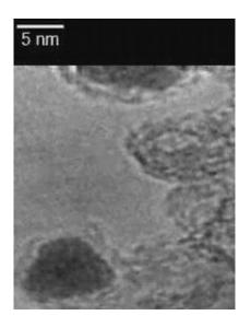
High-resolution transmission electron micrograph that reveals the possibility of platinum skin formation on nanoscale surfaces. Credit: Argonne National Laboratory
