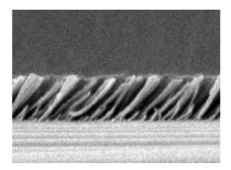
To achieve a very low refractive index, silica nanorods are deposited at an angle of precisely 45 degrees on top of a thin film of aluminum nitride. Credit: Rensselaer/Fred Schubert
