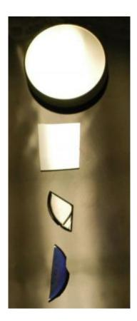
From top, light reflecting off surfaces made from aluminum, silicon, and aluminum nitride. At bottom is a piece of aluminum nitride coated with the new anti-reflection material. Credit: Rensselaer/Fred Schubert
