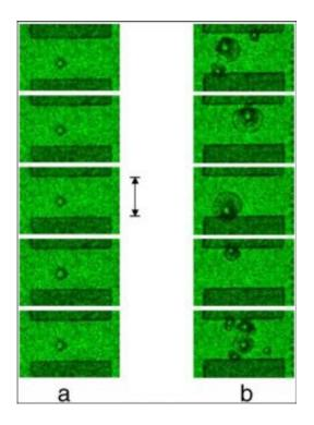
Ultra-highspeed photographs of microbubbles forming on a microheater show the effect of residual nanobubbles between heating pulses. The first pulse of a two-pulse sequence (a) produces nearly identical microbubbles time after time, but the second pulse (b) produces a random assortment of bubbles of varying sizes. Vertical bar shows a distance of 15 micrometers. Credit: NIST
