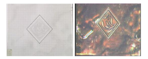
Images of a ceramic tile, taken with (left) a normal CCD, and (right) the multiangle scanner, showing detailed surface structure. Image reprinted with permission from Forrest, A. K. Copyright 2007, American Institute of Physics.
