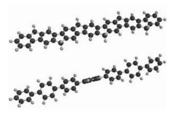
The reconstructed polymer (top) was found to conduct one thousand times better than the standard polymer (below) due to its fixed ladder-like structure. Credit: NWO
