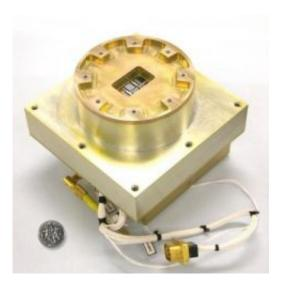
A close-up view of the Flat Plasma Spectrometer (FlaPS) shown next to a dime for scale. FlaPS was designed and fabricated by the Johns Hopkins University Applied Physics Laboratory for NASA and the US Air Force Academy. Credit: Johns Hopkins University Applied Physics Laboratory
