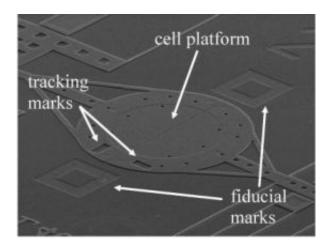
Electron micrograph of the NIST "cell puller," which measures the mechanical properties of a living cell. After the cell spreads and adheres to the center of the 200-micrometer-wide circular platform, half of the platform is pulled slowly away, while a sensor connected to the other half measures the force on the cell. Credit: D. Serrell/NIST
