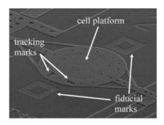
Electron micrograph of the NIST "cell puller," which measures the mechanical properties of a living cell. After the cell spreads and adheres to the center of the 200-micrometer-wide circular platform, half of the platform is pulled slowly away, while a sensor connected to the other half measures the force on the cell. Credit: D. Serrell/NIST
