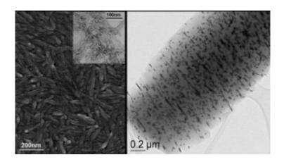
Left, an electron micrograph (TEM) of a metal, in this case platinum, deposited on cellulose. Inset, crystalline cellulose without metal. Right, TEM showing the pattern of platinum clustering along hydroxyl sites on the cellulose surface. Credit: Pacific Northwest National Laboratory
