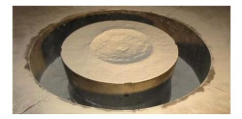
A 30cm-diameter crater plus spattered dust are all that's left after a test shot in the Ames Vertical Gun. Photo credit: NASA
