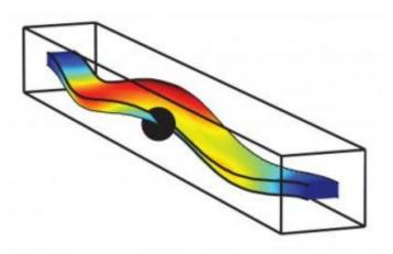
This slow-motion simulation of the JILA nanoscale motion detector shows the wiggling of a floppy metal beam, just 100 nanometers thick, as it is struck by an electric current at the dot. Red indicates the greatest change in position from the rest state. Credit: Credit: K. Lehnert/JILA
