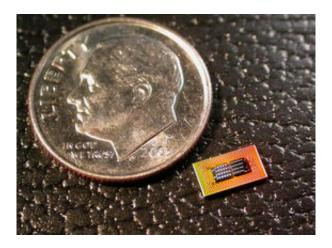
At the 2007 Optical Fiber Conference, IBM scientists will reveal a prototype optical transceiver chipset capable of reaching speeds at least eight times faster than optical components available today.
