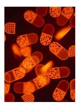
MIT researchers have developed a high-throughput method for the detection of biomolecules (such as DNA shown here) using multifunctional particles. The technique could make medical diagnostics and drug discovery faster and cheaper. Image / Daniel Pregibon
