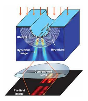
Schematic of an optical hyperlens that can magnify and project sub-diffractionlimited objects onto a far-field plane. The objects and the hyperlens are enlarged to show details; they are actually much smaller than a conventional lens. Images courtesy the Zhang Lab, UC Berkeley
