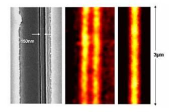
Hyperlens imaging of a pair of nanowires 35 nm wide and spaced 150 nm apart. On the left is a scanning electron microscope image of the lines. In the middle is the magnified hyperlens image showing the 150 nm spaced line pair. Without the hyperlens, the two lines cannot be distinguished, as in the image taken in a control experiment shown to the right. Images courtesy the Zhang Lab, UC Berkeley
