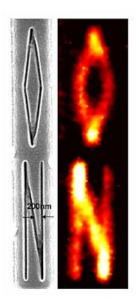
Shown on the left is a scanning electron microscope image of nanowires shaped in the letters O and N. To the right is the hyperlens image of the nanowires.
