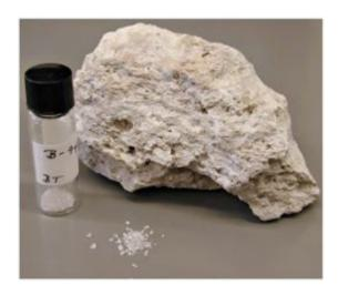
A piece of supervolcano and extracted quartz crystals analyzed for titanium. Credit: Rensselaer Polytechnic Institute/David Wark
