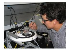
NIST chemist James Kushmerick adjusts test apparatus demonstrating a prototype silver nanoswitch. Credit: NIST
