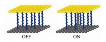
Silver nanoswitch: When the voltage between a gold conductor (top) and silver conductor (bottom) exceeds a critical point, silver ions rapidly assemble like a lightning strike to bridge the gap through a organic molecule monolayer. Credit: NIST
