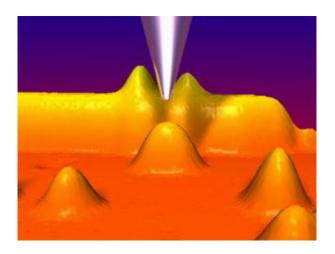
Artists view of the measurement set up with the metallic tip of the scanning tunnelling microscope on top of a chain made out of three cobalt adatoms on a copper surface. The bump to the left is a single cobalt atom. Credit: Max Planck Institute for Solid State Research
