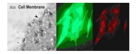
Nanotube length threshold: NIST experiments using human lung cells demonstrate that DNA-wrapped single-walled carbon nanotubes longer than about 200 nanometers are excluded from cells, while shorter lengths are able to penetrate the cell interior (dark lines in the fluorescence image above). Credit: NIST
