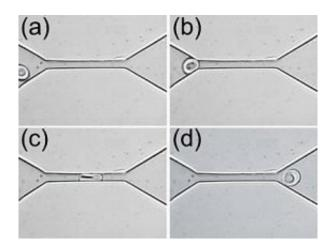
An experimental in vitro demonstration of the "fluidization" of a healthy human red blood cell through a microfliuidic channel at room temperature. The series of images shows how the shape of a red blood cell changes as it is squeezed through a 4 micron by 4 micron channel. Photo / David J. Quinn
