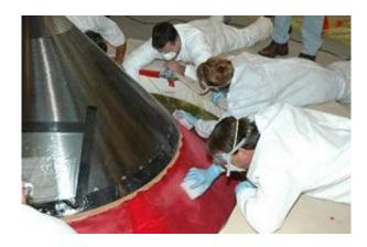
In highbay 1 inside the Vehicle Assembly Building, technicians begin to carefully sand away the red dye that has been applied to the external tank to help expose cracks or compression dents. Photo credit: NASA/Jim Grossman
