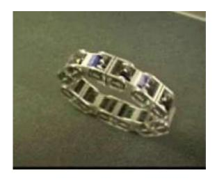
SuperBot modular robotic units assemble into a circular structure able to roll like a wheel. Credit: USC Information Sciences Institute
