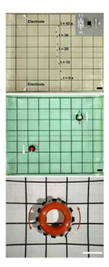
NC State&acutes tiny, self-propelling diodes move (top); move and light up (middle); and spin around (bottom) in liquid.
