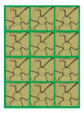
A colored montage of a ring oscillator used in the microfluidic computer developed by researchers at MIT. Starting with top left image, and reading left to right, the yellow bubble flows around the ring until it reaches and joins a stream of bubbles. Image / Felice Frankel and Manu Prakash, MIT
